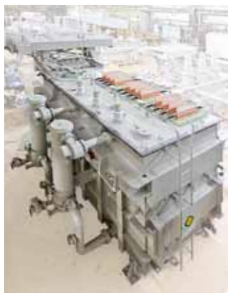
OFWF-60Hz-75 (90:OL) MVA-22.8kV \Delta -F1110 ~ R860 ~ 635V open \Delta (25V step 20taps)
