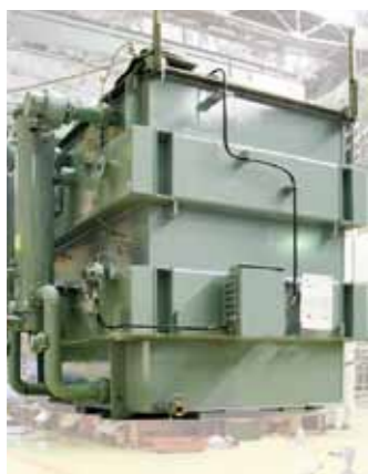
OFWF-60Hz-70 (84:OL) MVA-22kV \Delta -F1100 ~ R770 ~ 500V open \Delta (30V step 21taps)
